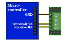
Figure 20. Wiring Between MotorController and Kangaroo
