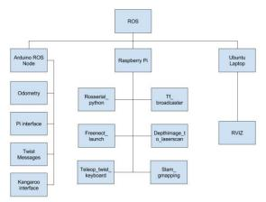
Figure 23. Software Block Diagram
