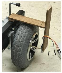
Figure 8. Mounting encoder onto wheelchair
