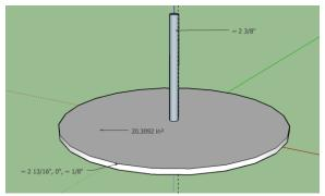
Figure 27.CAD Drawing of Encoder Adapter
