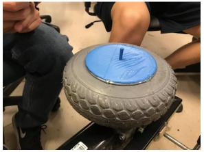
Figure 30. Encoder Adapter Mounted
