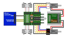
Figure 19. MotorController and Encoder Diagram
